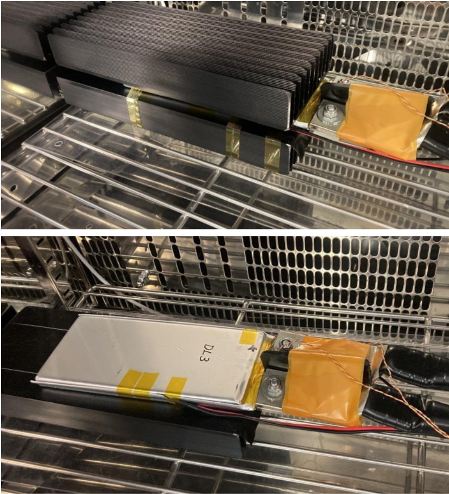
Figure 1. Cell was placed between heat sinks (top image, two-sided heat sink) or on top of a single heat sink (bottom image, one-sided heat sink), with temperature sensors attached to the tabs and under the folded seam on the side.
